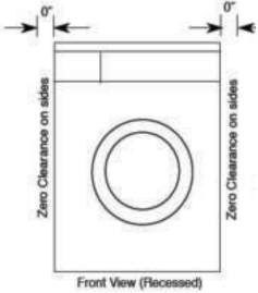
If the appliance is to be installed in a closet, the installation must be completed by a qualified person or service representative. Adequete blocking to secure unit is required.
